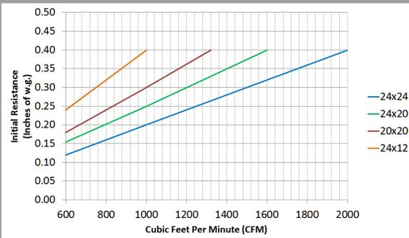
Initial resistance versus airflow, recommended velocity is 400 feet per minute or less to obtain published adsorbent efficiency.
